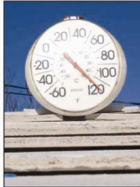
ROOF TEMPERATURE READING OUTSIDE AS OF 02-04-07 12:30 PM =119 °F
